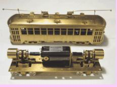
broken in and lubricated. We feel that that placement of the flywheels may be a problem. Currently accepted practice is to mount flywheels on the motor shaft, otherwise they tend to emit a vibration which translates to noise, especially at higher operating speeds.
